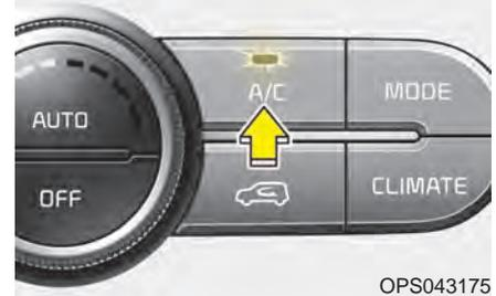
Push the A/C button to turn the air conditioning system on (indicator light will illuminate).
