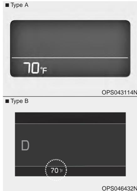
This gauge indicates the current outside air temperatures by 1°F (1°C).
