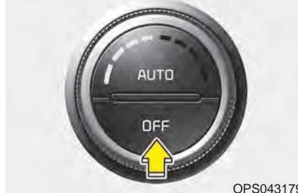
Push the OFF button to turn off the blower. However you can still operate the mode and air intake buttons as long as the ignition switch is in the position ON.
