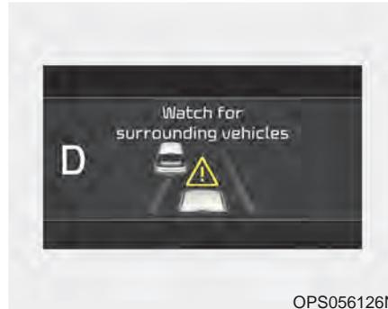
If the vehicle ahead (vehicle speed: less than 20 mph (30 km/h)) moves to the next lane, the warning chime will sound and a message will appear.
