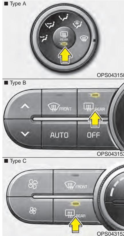
The defroster heats the window to remove frost, fog and thin ice from the rear window, while the engine is running.
