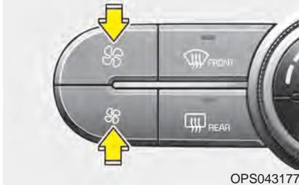
The fan speed can be set to the desired speed by pressing the fan speed control button.
