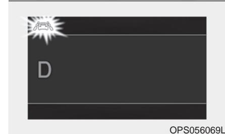
When the LDWS is not working properly, the warning light will illuminate and the warning message will come on for a few seconds. After the message disappears, the master warning light will illuminate.
