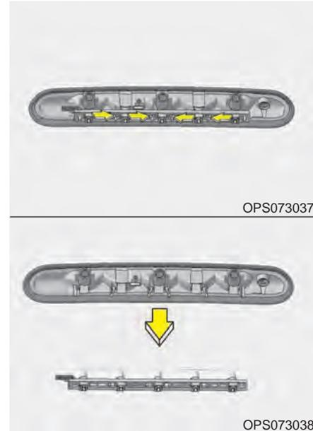
4. Pull out the module from the high mounted stop lamp assembly by pulling both clips.
