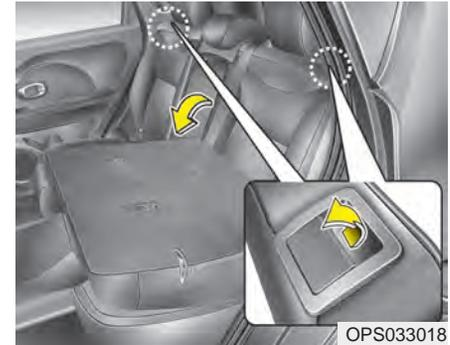
4. Pull on the seatback folding lever, then fold the seat toward the front of the vehicle. When you return the seatback to its upright position, always be sure it has locked into position by pushing on the top of the seatback.
