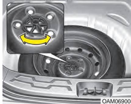
Turn the tire hold-down wing bolt counterclockwise.
