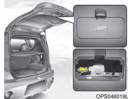
Your vehicle is equipped with an emergency liftgate safety release lever located on the bottom of the liftgate. When someone is inadvertently locked in the compartment. The liftgate can be opened by doing as follows:
