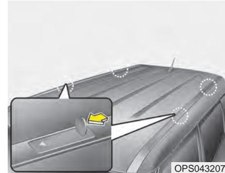
To install or remove a roof carrier, you can use the mounting bracket and cover on the roof.
