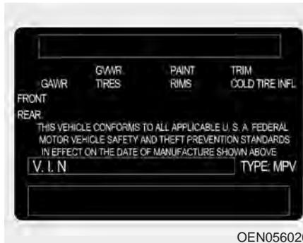
The certification label is located on the driver's door sill at the center pillar.
