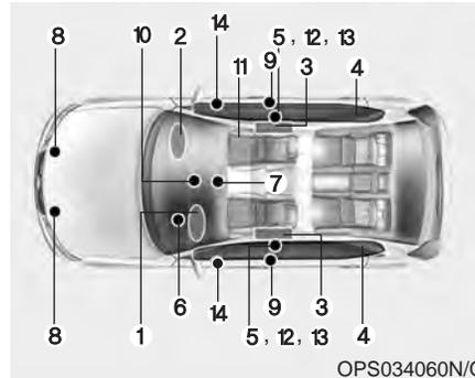
The SRS consists of the following components:
