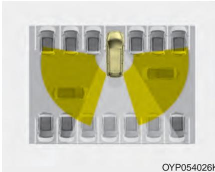
When your vehicle moves backwards from a parking position, the sensor detects approaching vehicles to the left or right side direction and gives information to the driver.
