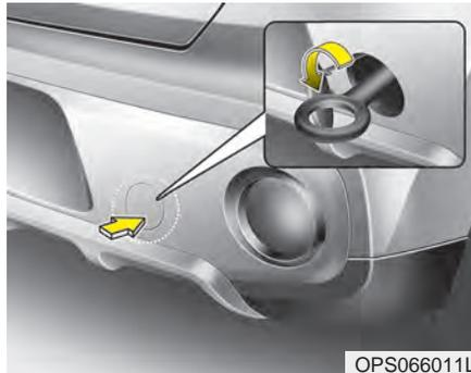
3. Install the towing hook by turning it clockwise into the hole until it is fully secured.
