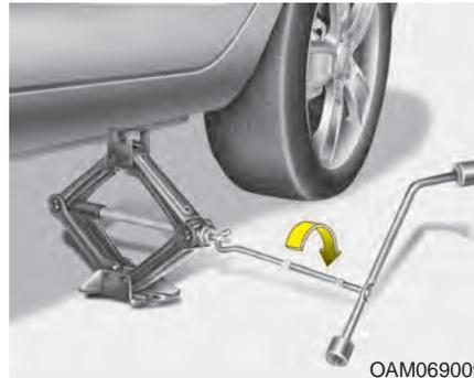
8. Insert the jack handle into the jack and turn it clockwise, raising the vehicle until the tire just clears the ground. This measurement is approximately 1 in. (30 mm).
