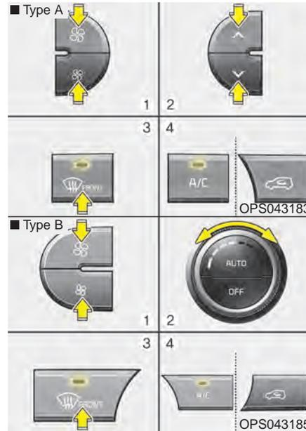
1. Set the fan speed to the desired position.
