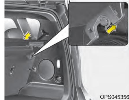
3. While lifting the cover up, hold the area near the front slots. Then, pull up the cover at approximately 45° angle.
