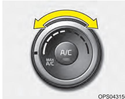
The temperature control knob allows you to control the temperature of the air flow from the ventilation system. To change the air temperature in the passenger compartment, turn the knob to the right position for warm air or left position for cooler air.
