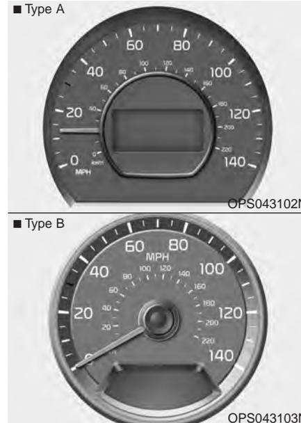
The speedometer indicates the speed of the vehicle and is calibrated in miles per hour (mph) and/or kilometers per hour (km/h).
