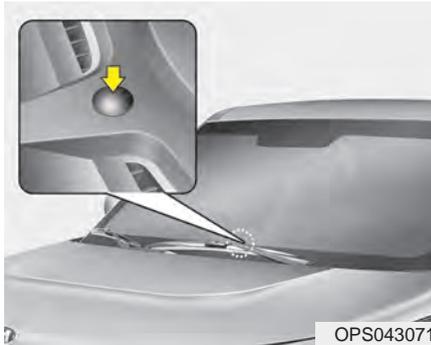
Never place anything over the sensor located on the instrument panel to ensure better control of the heating and cooling system.
