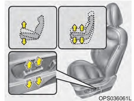
Pull the front portion of the control switch up to raise or press down to lower the front part of the seat cushion. Pull the rear portion of the control switch up to raise or press down to lower the seat cushion. Release the switch once the seat reaches the desired position.
