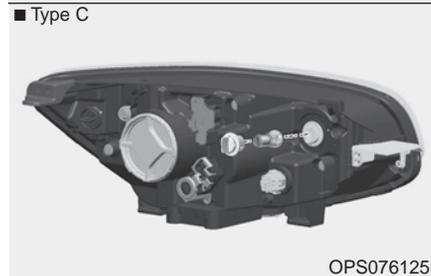
6. Remove the socket from the assembly by turning the socket counterclockwise until the tabs on the socket align with the slots on the assembly.
