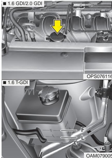
If the coolant level is low, add enough specified coolant to provide protection against freezing and corrosion. Bring the level to F, but do not overfill. If frequent additions are required, see an authorized Kia dealer for a cooling system inspection.
