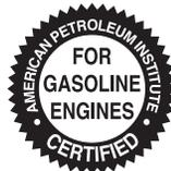
\*1: An engine oil displaying this API Certification Mark conforms to the international Lubricant Specification Advisory Committee (ILSAC). It is recommended to only use engine oils that uphold this API Certification Mark.
