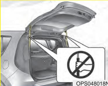
Do not hold the part (gas lifter) that supports the tailgate. Be aware that the deformation of the part may cause vehicle damage and a risk of injury.
