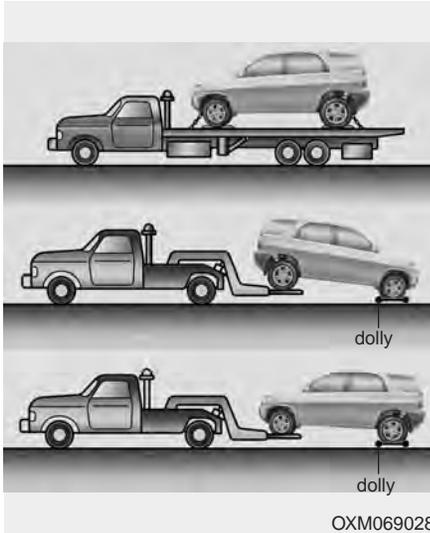
If emergency towing is necessary, we recommend having it done by an authorized Kia dealer or a commercial tow-truck service. Proper lifting and towing procedures are necessary to prevent damage to the vehicle. The use of wheel dollies or flatbed is recommended.
