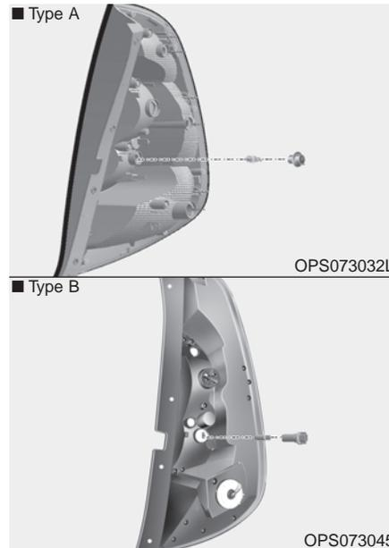
4. Remove the socket from the assembly by turning the socket counterclockwise until the tabs on the socket align with the slots on the assembly.
