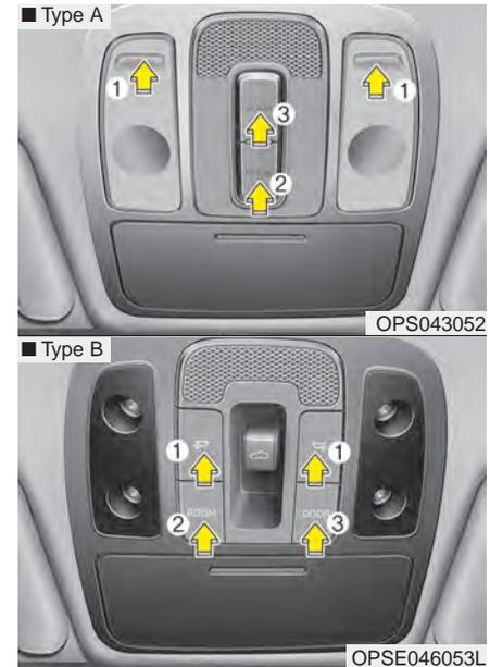
Press the lens (1) or button (1) to turn the map lamp on or off
