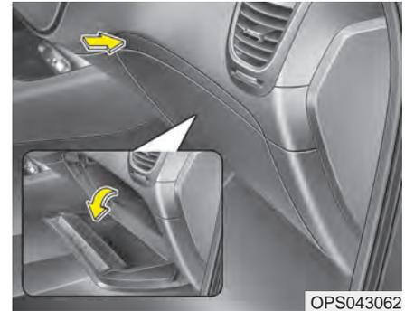
To open the glove box, push the button and the glove box will automatically open. Close the glove box after use.
