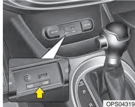
If your vehicle has an AUX and/or USB (universal serial bus) port, you can use an AUX port to connect audio devices and an USB port to plug in a USB.
