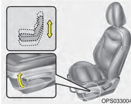
To change the height of the seat, push the lever upwards or downwards.
