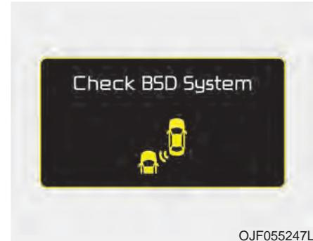
If the system does not work properly, a warning message will appear and the light on the switch will turn off. The system will turn off automatically.
