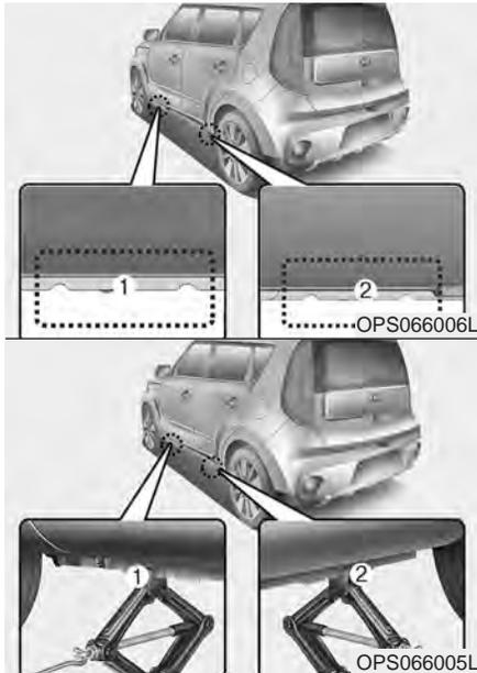
7. Place the jack at the front (1) or rear (2) jacking position closest to the tire you are changing. Place the jack at the designated locations under the frame.
