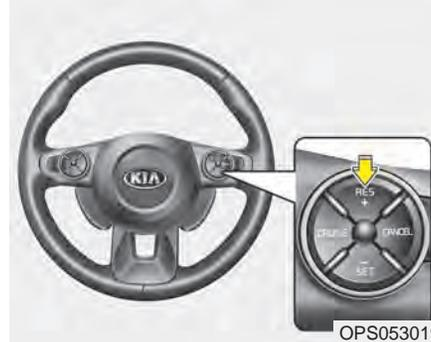
If any method other than the CRUISE button was used to cancel cruising speed and the system is still activated, the cruising speed will automatically resume when you move the lever up/down (to RES+ or SET-).
