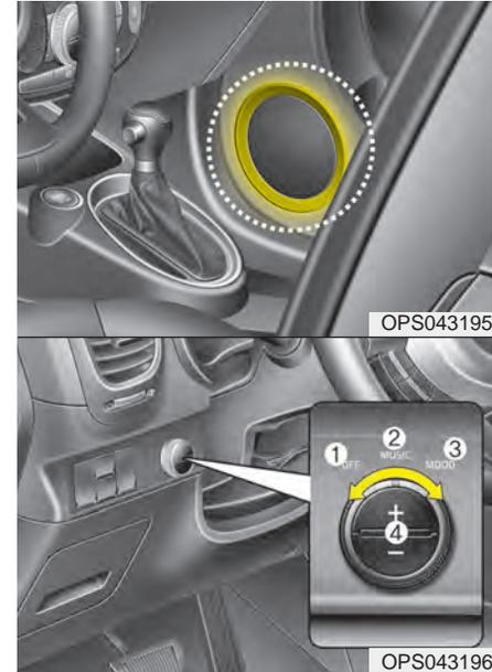
The speaker lights that light around the front speaker are adjusted by turning the knob as follows.
