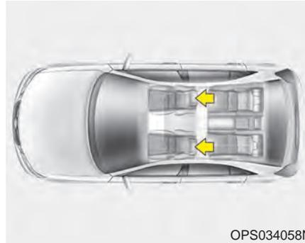
The driver's and front passenger's seats are equipped with a headrest for the occupant's safety and comfort. The headrest not only provides comfort for the driver and front passenger, but also helps protect the head and neck in the event of a rear collision.
