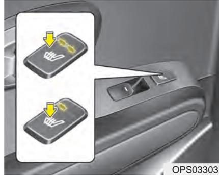
The seat warmer is provided to warm the rear outboard seats during cold weather. With the ignition switch in the ON position, push either of the switches to warm rear seats.
