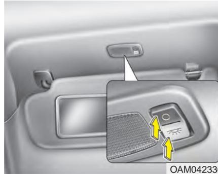
Pull the sunvisor downward and you can turn the vanity mirror lamp ON or OFF by pushing the button.
