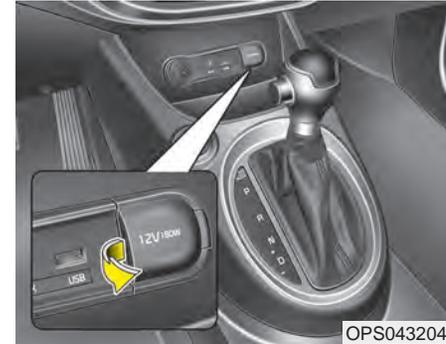
8. Plug the compressor power cord into the front passenger side power outlet of the vehicle.
