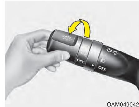
When the light switch is in the headlight position (2nd position), the head, tail, license and instrument panel lights will turn ON.
