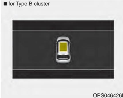
If the driver removes the ignition key (smart key: turns off the engine) when the sunroof is not fully closed, the warning chime will sound for a few seconds and a message will appear on the LCD display or warning indicator will illuminate.
