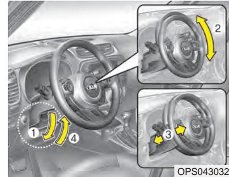
To change the steering wheel angle, pull down the lock-release lever (1), adjust the steering wheel to the desired angle (2) and height (3, if equipped) then pull up the lock-release lever to lock (4) the steering wheel in place. Be sure to adjust the steering wheel to the desired position before driving.
