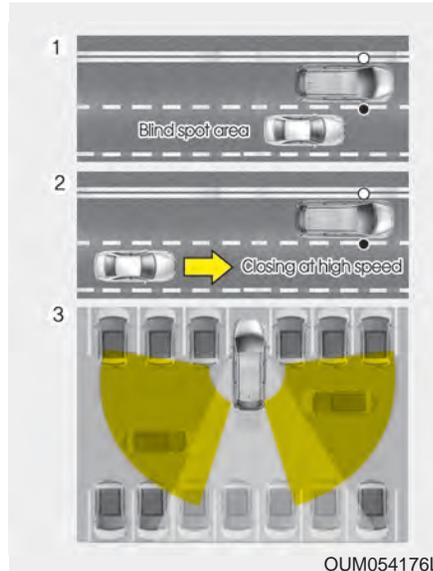
The BSD (Blind spot detection) system uses a radar sensor to alert the driver while driving.
