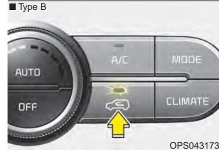
This is used to select outside (fresh) air position or recirculated air position.
