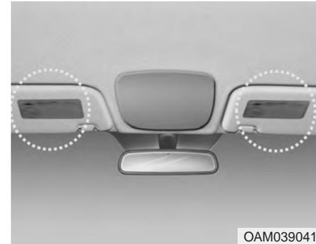
Air bag warning labels, some required by the U.S. National Highway Traffic Safety Administration (NHTSA), are attached to the sunvisor to alert the driver and passengers of potential risks of the air bag system.
