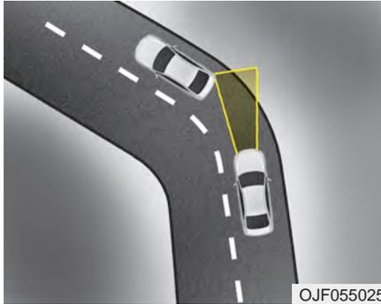
The SCC may have limits to its ability to detect distance to the vehicle ahead due to road and traffic conditions.
