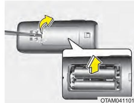
When replacement is necessary, use the following procedure.
