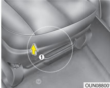
The vehicle identification number (VIN) is the number used in registering your vehicle and in all legal matters pertaining to its ownership, etc. The number is punched on the floor under the front passenger seat. To check the number, remove the cover (1).
