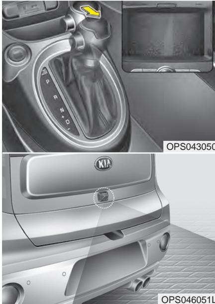
This system is a supplemental system that helps the driver by displaying objects behind the vehicle when backing up.
