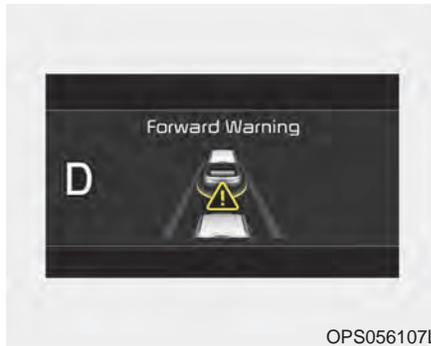
The warning message appears on the LCD display with the warning alarms.
