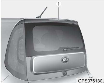
If the High mounted stop lamp (LED type) (1) does not operate, we recommend that you have your vehicle checked by an authorized Kia dealer.
