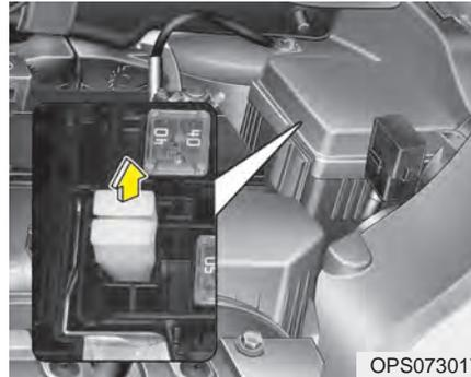
3. Pull the suspected fuse straight out. Use the fuse puller provided on the engine compartment fuse panel cover.
