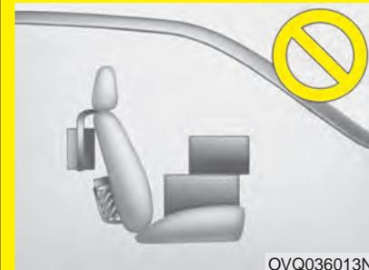
**- Do not place heavy loads in the front passenger seatback pocket or on the front passenger seat.**
