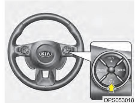
3. Push the SET - switch, and release it at the desired speed. The SET indicator light in the instrument cluster will illuminate. Release the accelerator pedal at the same time. The desired speed will automatically be maintained.
