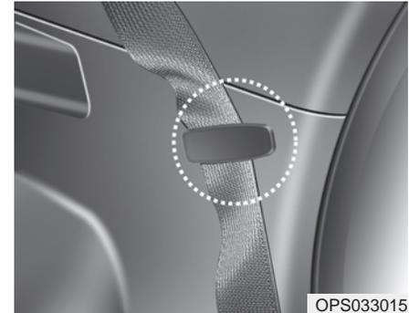
Routing the seat belt webbing through the rear seat belt guides will help keep the belts from being trapped behind or under the seats.
