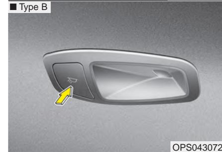
Press the button to turn the light on or off.
