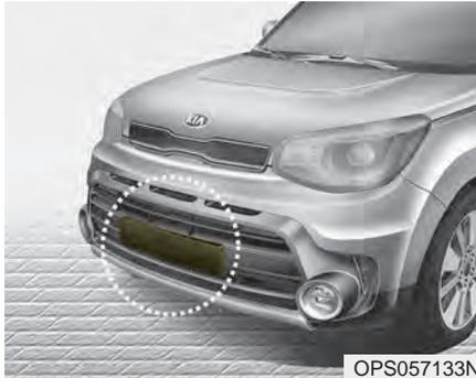
The sensor detects the distance to the vehicle in front. However, a foreign substance on the sensor lens, such as snow and rain, may adversely affect the sensing performance. It may even temporarily cancel the AEB. Always keep the sensor lens clean.
