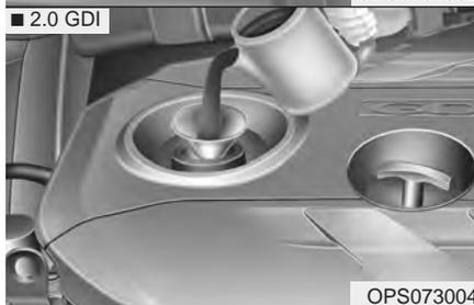
If it is near or at L, add enough oil to bring the level to F. **Do not overfill.**
