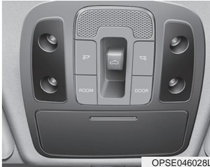
The sunroof can be operated for approximately 30 seconds after the ignition key is removed or turned to the ACC or LOCK position. However, if the front doors are opened, the sunroof cannot be opened even within the 30 seconds period.
