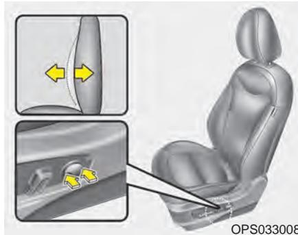
The depth of the lumbar support can be adjusted by pressing the button fore and after. If equipped, the location of the lumbar support can be adjusted up and down by pressing the button up and down.
