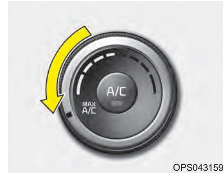
To operate the MAX A/C, turn the temperature knob to extreme left. Air flow is directed toward the upper body and face.
