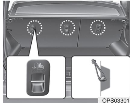
First secure the child restraint with the LATCH lower anchors or the seat belt. If the child restraint manufacturer recommends that the top tether strap be attached, attach and tighten the top tether strap to the top tether anchor.
