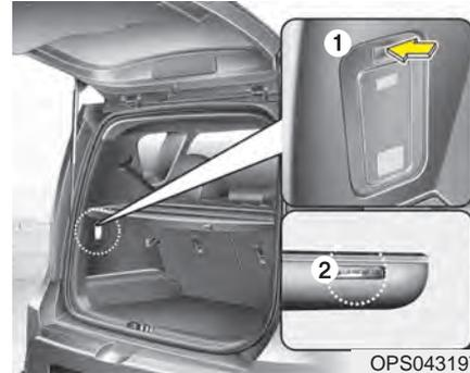
In-vehicle lamp, if necessary, after separation can be used as a portable.
