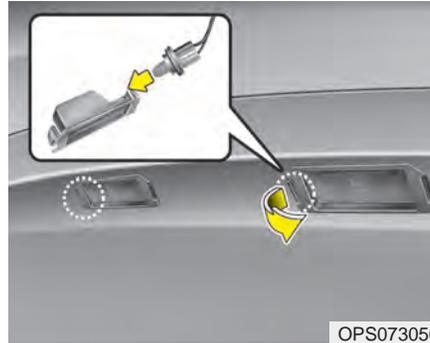
1. Remove the lens by pressing the tabs.
