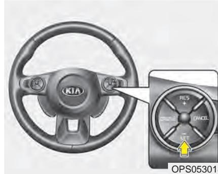
3. Move the lever down (to SET-), and release it at the desired speed. The set speed and vehicle to vehicle distance on the LDC screen will illuminate.
