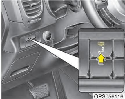
The indicator on the switch will illuminate when the BSD (Blind spot detection) system switch is pressed with the engine start/stop button ON. If the vehicle speed exceeds 18.6 mph (30 km/h), the system will activate.
