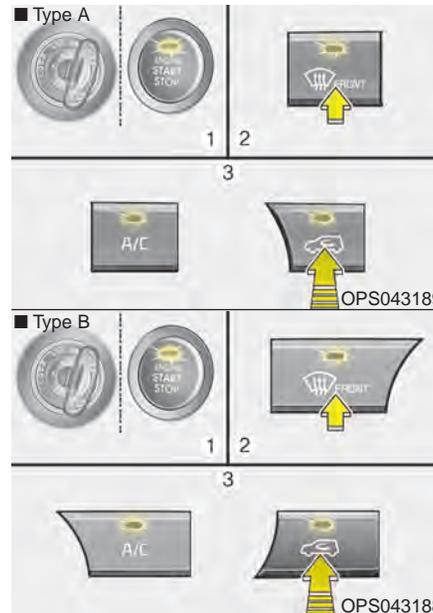
1. Turn the ignition switch to the ON position.
