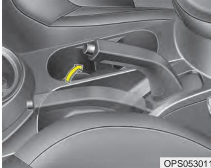
To engage the parking brake, first apply the foot brake and then without pressing the release button in, pull the parking brake lever up as far as possible.
