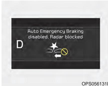
When the sensor is covered or the sensor lens is dirty with foreign substances, such as snow or rain, the AEB operation may temporarily stop. In this case, a warning message will appear to notify the driver.
