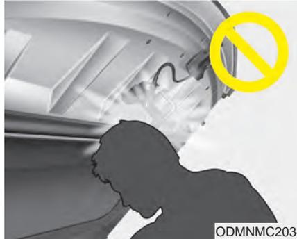
When you check the engine compartment, take caution to avoid contacting your head with the safety hook which is located inside of the hood.
