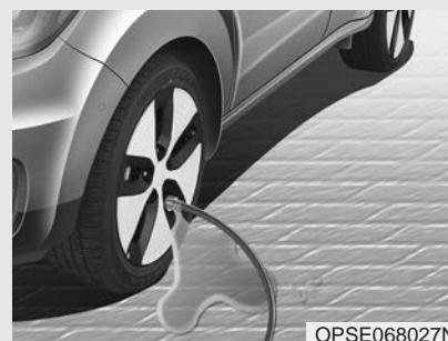
*Securely install the sealant filling hose to the valve. If not, sealant may flow backward, possibly clogging the filling hose.*
