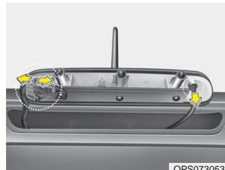
4. Pull out the module from the high mounted stop light assembly by pulling both clips.
