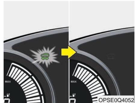
5. Check if the indicator lamp (car icon) is turned OFF on the instrument cluster.
