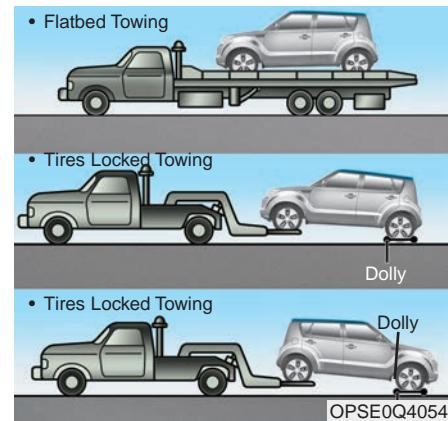
If towing is required, lift all four wheels off the ground and tow the vehicle. If you must tow the vehicle using only two wheels, lift the front wheels off the ground and tow the vehicle.
