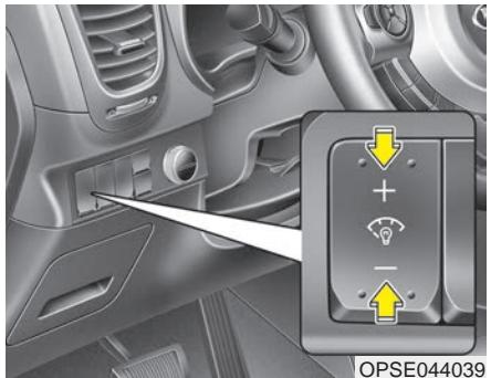
The brightness of the instrument panel illumination is changed by pressing the illumination control button ("+" or "-") when the POWER button is ON, or the tail lights are turned on.
