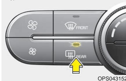
To activate the rear window defroster, press the rear window defroster button located in the center facia switch panel.
