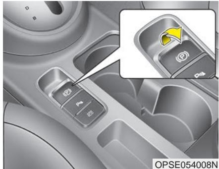
To apply the EPB (electronic parking brake):
