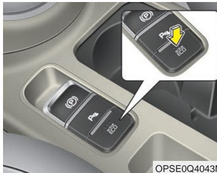
Active ECO helps improve energy efficiency by controlling certain motor and climate control system operating parameters. Energy efficiency depends on the driver's driving habit and road condition.
