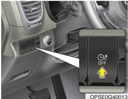
To immediately charge the battery (not at reserved time only) first connect the charging cables. Then, the Deactivate Reserved Charge button [
