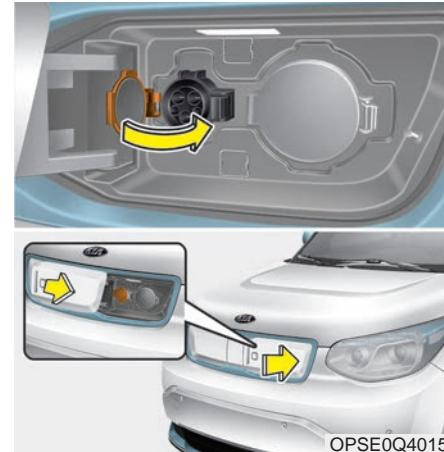
3. Make sure to completely close the normal charging inlet cover.
