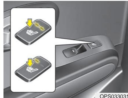
The seat warmer is provided to warm the rear outboard seats during cold weather. With the POWER button in the ON position, push either of the switches to warm rear seats.
