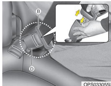
Press the release button on the buckle (D) and remove the tongue plate (B) from the buckle (D).
