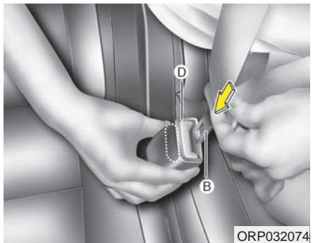
2. Pull the tongue plate (B) and insert the tongue plate (B) into the open end of the buckle (D) until an audible "click" is heard, indicating the latch is locked. Make sure the belt is not twisted.
