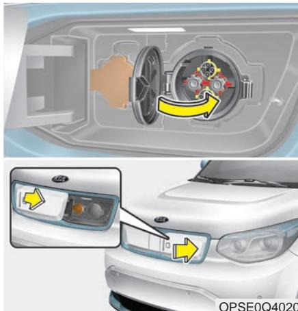
2. Make sure to completely close the quick charging inlet cover.
