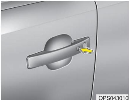
The button will only operate when the smart key is within 0.7~1m (28~40 in.) from the outside door handle.
