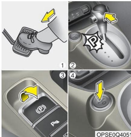
1. Hold down the brake pedal while the vehicle is parked.
