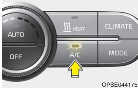
Push the A/C button to turn the air conditioning system on (indicator light will illuminate).
