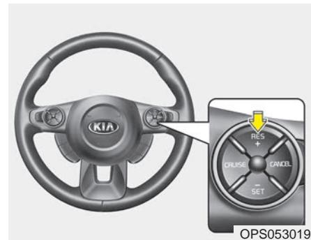
If any method other than the CRUISE button was used to cancel cruising speed and the system is still activated, the most recent set speed will automatically resume when the RES+ switch is pushed.
