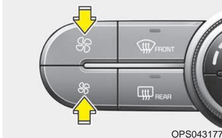
To change the fan speed, press the button (♣) for higher speed, or push the button (♦) for lower speed. To turn the fan speed control off, press the OFF button and select outside (fresh) air position.
