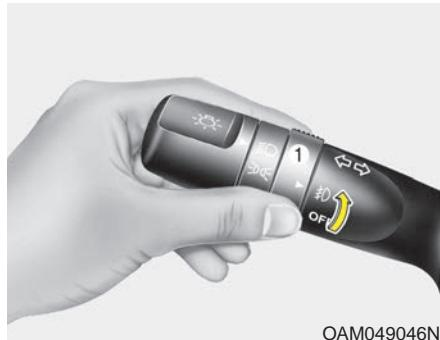
Fog lights are used to provide improved visibility when visibility is poor due to fog, rain or snow, etc. The fog lights will turn on when the fog light switch (1) is turned to the on position after the headlight is turned on.
