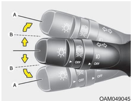
The POWER button must be on for the turn signals to function. To turn on the turn signals, move the lever up or down (A). The green arrow indicators on the instrument panel indicate which turn signal is operating. They will self-cancel after a turn is completed. If the indicator continues to flash after a turn, manually return the lever to the OFF position.
