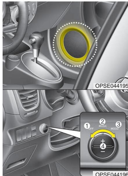
The speaker lights that lights around the front speaker is adjusted by turning the knob as follows.
