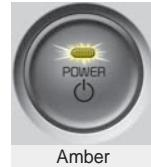
To turn off the vehicle, press the POWER button with the shift lever in the P (Park) position. When you press the POWER button without the shift lever in the P (Park) position, the POWER button will not change to the OFF position but to the ACC position.
