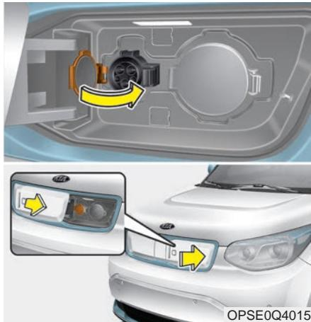
3. Make sure to completely close the normal charging inlet cover.
