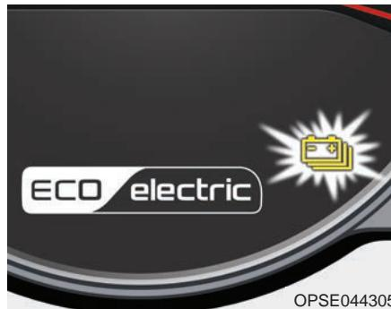
When there are 3 gauge bars (near the "MIN" area) on the high voltage charge indicator, the warning lamp turns ON to alert you of the battery level.
