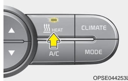
Push the HEAT button to turn the heater on (indicator light will illuminate). Push the button again to turn the heater off.
