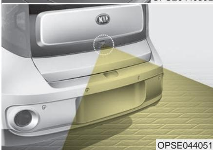
The rear view monitor will activate when the back-up light is ON with the POWER button ON and the shift lever in the R (Reverse) position
