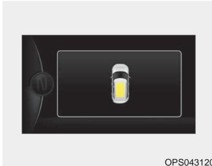
If the driver removes the ignition key (smart key: turns off the engine) when the sunroof is not fully closed, the warning chime will sound for a few seconds and a message will appear on the LCD display or warning indicator will illuminate.
