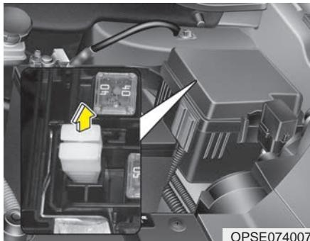
3. Pull the suspected fuse straight out. Use the fuse puller provided on the motor compartment fuse panel cover.
