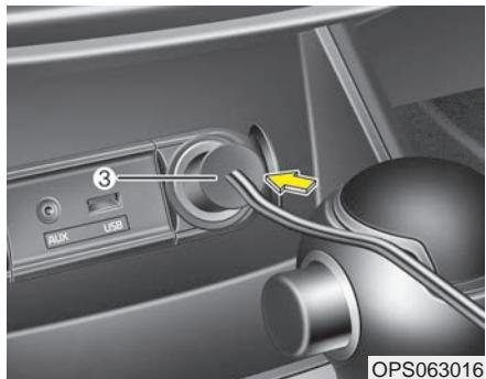
7. Plug the compressor power cord (3) into the front passenger side power outlet (180W) of the vehicle.
