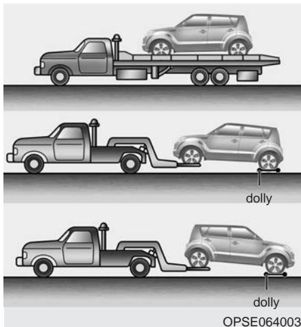
If emergency towing is necessary, we recommend having it done by an authorized Kia dealer or a commercial tow-truck service. Proper lifting and towing procedures are necessary to prevent damage to the vehicle. The use of wheel dollies or flatbed is recommended.
