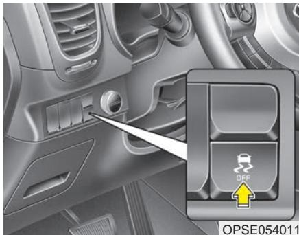
The Electronic Stability control (ESC) system is designed to stabilize the vehicle during cornering maneuvers. ESC checks where you are steering and where the vehicle is actually going. ESC applies the brakes on individual wheels to stabilize the vehicle.
