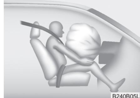
Upon deployment, tear seams molded directly into the pad covers will separate under pressure from the expansion of the air bags. Further opening of the covers then allows full inflation of the air bags.
