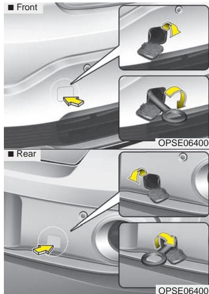
3. Install the towing hook by turning it clockwise into the hole until it is fully secured.
