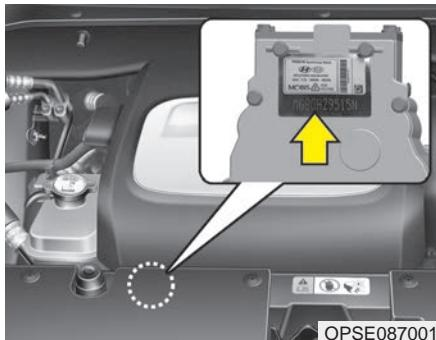
The motor number is stamped on the motor compartment as shown in the drawing.
