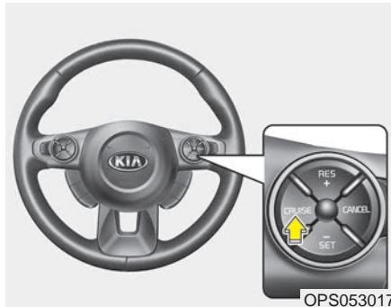
1. Press the CRUISE button on the steering wheel to turn the system on. The CRUISE indicator light in the instrument cluster will illuminate. Release the accelerator pedal at the same time. The desired speed will automatically be maintained.
