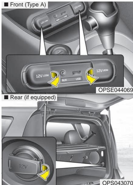
The power outlet is designed to provide power for mobile telephones or other devices designed to operate with vehicle electrical systems.
