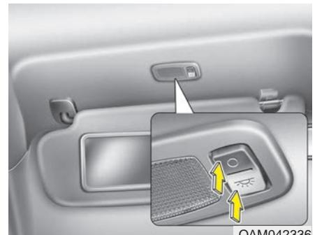
Pull the sunvisor downward and you can turn the vanity mirror lamp ON or OFF by pushing the button.
