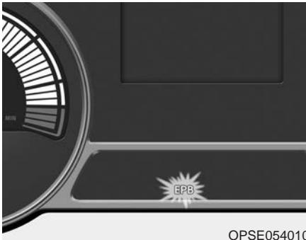
This warning light illuminates if the POWER button is changed to the ON position and goes off in approximately 3 seconds if the system is operating normally.
