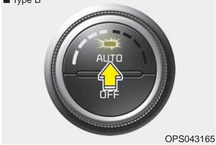
1. Push the AUTO button. It is indicated by AUTO on the display. The modes, fan speeds, air intake, air-conditioning and heater will be controlled automatically by temperature setting.
