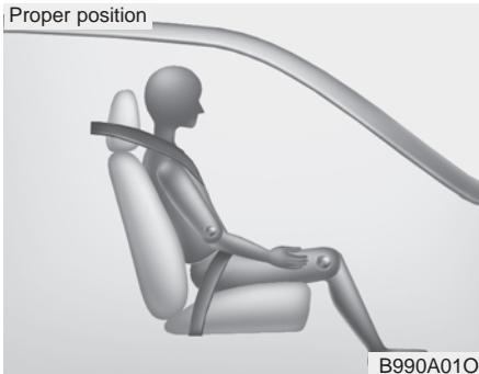
When an adult is seated in the front passenger seat, if the PASSENGER AIR BAG "OFF" indicator is on, turn the vehicle off and ask the passenger to sit properly (sitting upright with the seat back in an upright position, centered on the seat cushion with their seat belt on, legs comfortably extended and their feet on the floor). Restart the vehicle and have the person remain in that position. This will allow the system to detect the person and to enable the passenger air bag.
