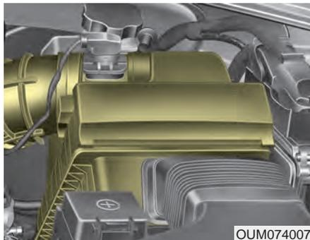
It must be replaced when necessary, and should not be washed.
