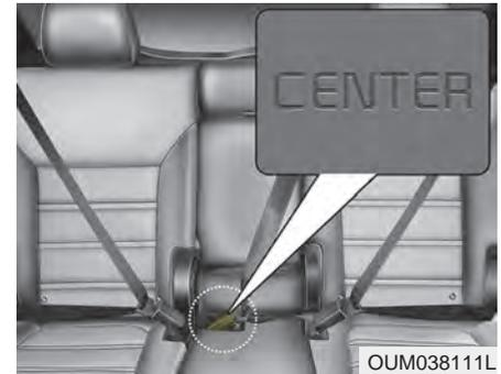
When using the rear center seat belt, the buckle with the “CENTER” mark must be used.
