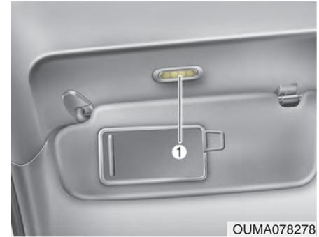
If the vanity mirror lamp (LED) (1) does not operate, have the vehicle checked by an authorized Kia dealer. The LED lamps cannot be replaced as a single unit because it is an integrated unit. The LED lamps has to be replaced with the unit.
