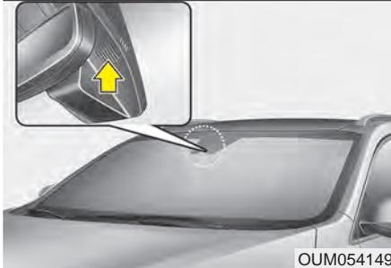
The Lane Keeping Assist System detects the lane markers on the road with a front view camera at the front windshield, and assists the driver's steering to help keep the vehicle in the lanes.
