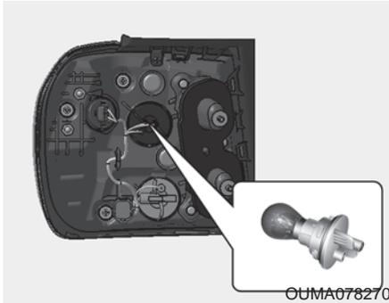
6. Remove the socket from the assembly by turning the socket counterclockwise until the tabs on the socket align with the slots on the assembly.
