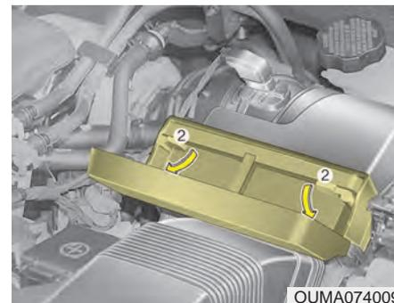
2. Unlock by turning the locking lever upward.
