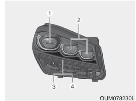
If the Low/High beam lamp(1,2), Front turn signal lamp(3), Day time running lamp/Position lamp(4) does not operate, have the vehicle checked by an authorized Kia dealer.
