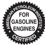
An engine oil displaying this API Certification Mark conforms to the international Lubricant Specification Advisory Committee (ILSAC). It is recommended to only use engine oils that uphold this API Certification Mark.
