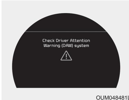
When the “Check System” warning message appears, the system is not working properly. In this case, have the vehicle inspected by an authorized Kia dealer.
