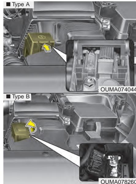
If the main fuse is blown, it must be removed as follows:
