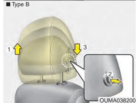
To raise the headrest, pull it up to the desired position (1). To lower the headrest, push and hold the release button (2) on the headrest support and lower the headrest to the desired position (3).
