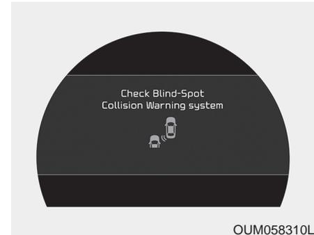
If the system does not work properly, a warning message will appear and the light on the switch will turn off. The system will turn off automatically.
