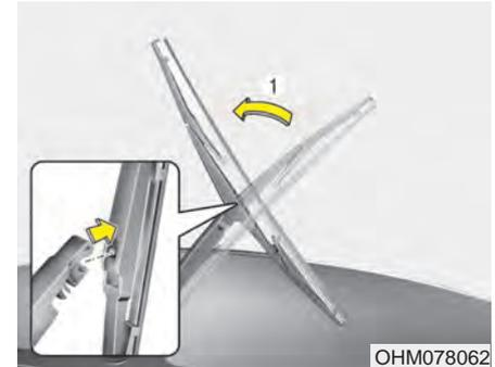
1. Raise the wiper arm and pull out the wiper blade assembly.
