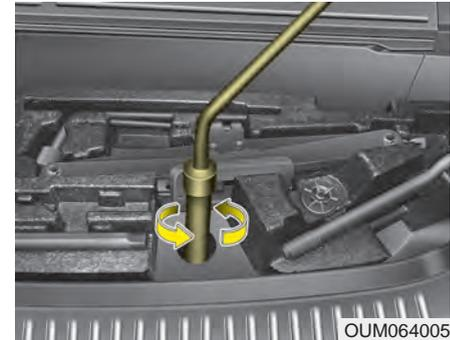
3. Connect the socket and wheel lug nut wrench.
