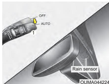
The rain sensor located on the upper end of the windshield glass senses the amount of rainfall and controls the wiping cycle for the proper interval. The more it rains, the faster the wiper operates. When the rain stops, the wipers stop.
