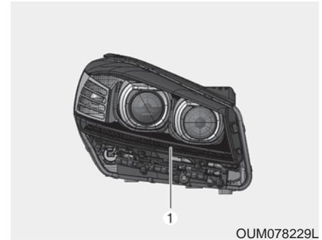
If the position lamp (LED) (1) does not operate, have the vehicle checked by an authorized Kia dealer. The LED lamps cannot be replaced as a single unit because it is an integrated unit. The LED lamps has to be replaced with the unit. A skilled technician should check or repair the position lamp (LED), for it may damage related parts of the vehicle.
