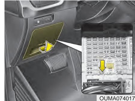
Always, put the fuse switch at the ON position.
