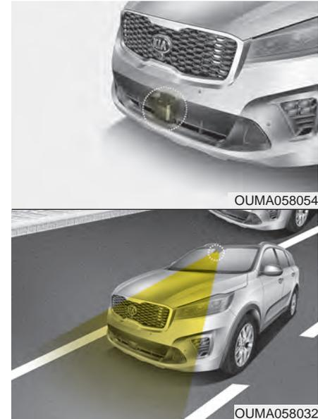
In order for the FCA system to operate properly, always make sure the sensor or sensor cover is clean and free of dirt, snow, and debris. Dirt, snow, or foreign substances on the lens may adversely affect the sensing performance of the sensor.
