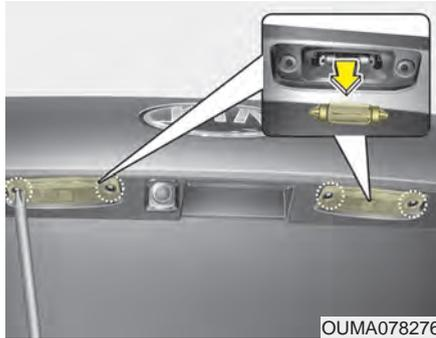
1. Remove the lamp cover by using a screwdriver.
