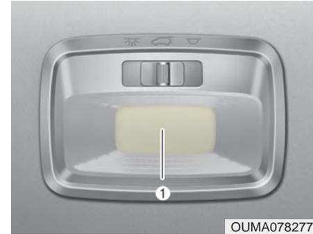
If the luggage lamp (LED) (1) does not operate, have the vehicle checked by an authorized Kia dealer. The LED lamps cannot be replaced as a single unit because it is an integrated unit. The LED lamps has to be replaced with the unit.
