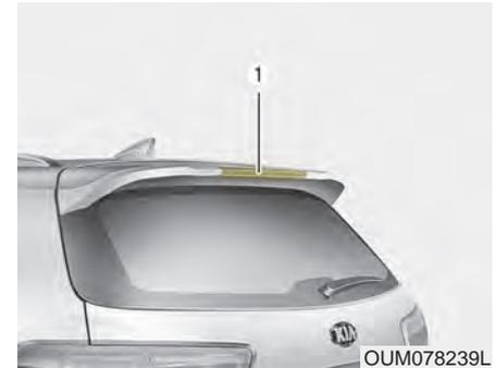
If the high mounted stop lamp (LED) (1) does not operate, have the vehicle checked by an authorized Kia dealer.
