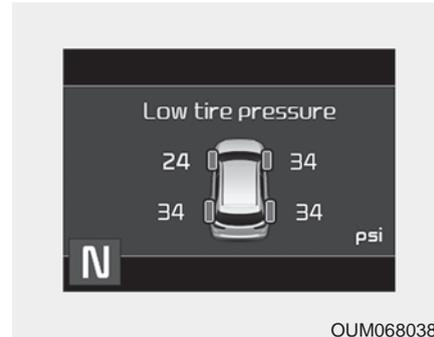
When the tire pressure monitoring system warning indicators are illuminated, one or more of your tires is significantly under-inflated.
