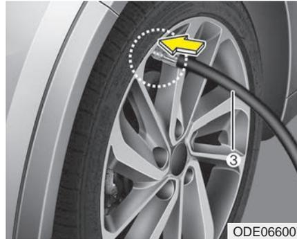
4. Unscrew the valve cap from the valve of the defective wheel and screw filling hose (3) of the sealant bottle onto the valve.
