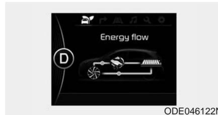
Electric and Engine power are used to move the vehicle.
