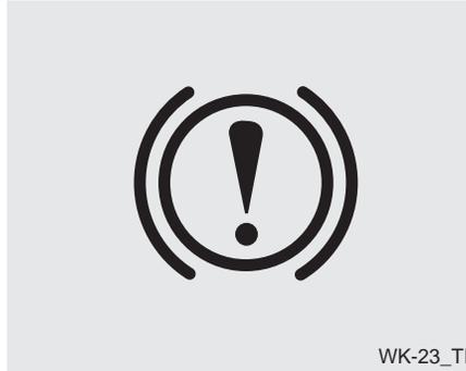
Check the brake warning light by pressing engine start/stop button ON (do not start the engine). This light will be illuminated when the parking brake is applied with the engine start/stop button in the START or ON position.
