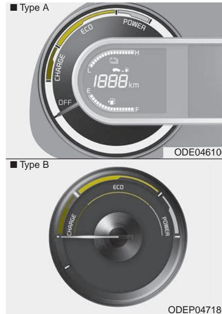
The hybrid system gauge indicates whether the current driving condition is fuel efficient or not.
