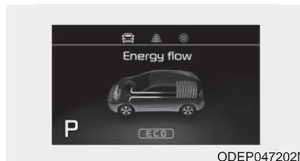
Electric power is used to move the vehicle.
