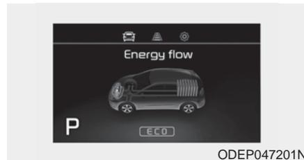
This mode means the vehicle has stopped.
