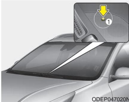
You can check the charging status from outside of vehicle when charging the high-voltage battery.
