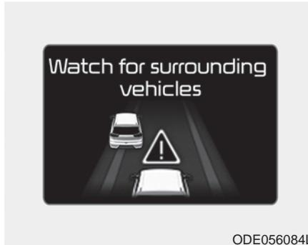
If the vehicle ahead (vehicle speed: less than 30 km/h (20 mph)) moves to the next lane, the warning chime will sound and a message will appear.
