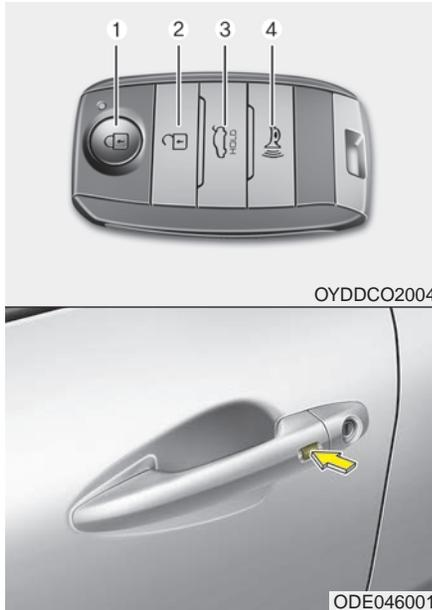
Pressing the button of the front outside door handles with all doors (and liftgate) closed and any door unlocked, locks all the doors (and liftgate).
