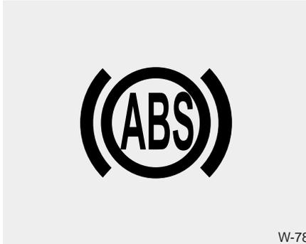
The ABS warning light will stay on for approximately 3 seconds after the engine start/stop button is ON. During that time, the ABS will go through self-diagnosis and the light will go off if everything is normal. If the light stays on, you may have a problem with your ABS. Contact an authorized Kia dealer as soon as possible.
