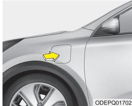
3. After unlocking doors, open the charging door by pressing it.
