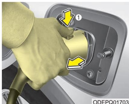
2. While holding the charging connector, pressing the locking release button(1) and then pull it out.
