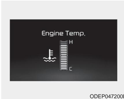
This gauge indicates the temperature of the engine coolant when the engine is running.
