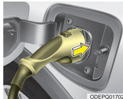
4. Remove any dust on the charging connector and charging inlet.
