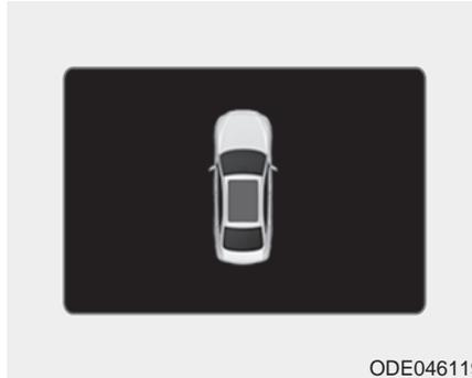
If the driver removes the ignition key (smart key: turns off the engine) when the sunroof is not fully closed, the warning chime will sound for a few seconds and a warning image will appear on the LCD window.
