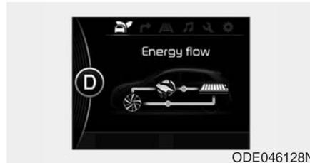
The vehicle is being slowed by engine compression and regenerative braking. The hybrid battery is being charged by regenerative braking.
