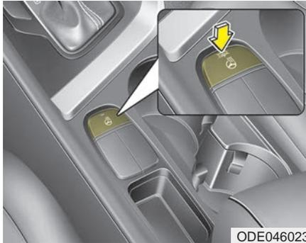
With the Engine Start/Stop button in the ON position, pressing the heated steering wheel button warms the steering wheel. The indicator on the button will illuminate.
