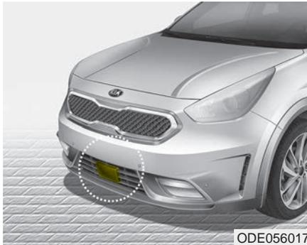
In order the AEB system to operate properly, always make sure the sensor is clean and free of dirt, snow, and debris. Dirt, snow, or foreign substances on the lens may adversely affect the sensing performance of the sensor. It may even temporarily cancel the AEB. Always keep the sensor lens clean.
