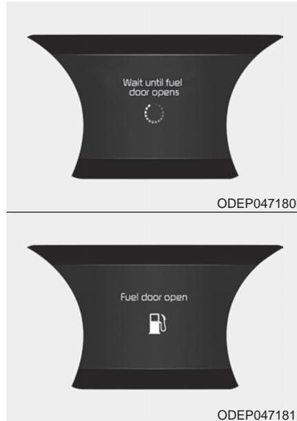
Wait until the fuel tank is depressurized. The message is displayed when the fuel filler lid opens after the fuel tank is depressurized.
