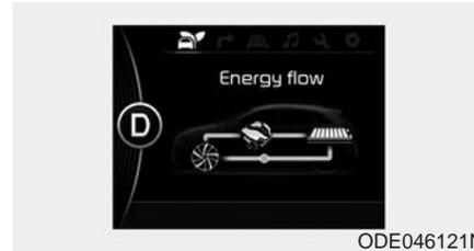
Electric power is used to move the vehicle. (Battery → Wheel)
