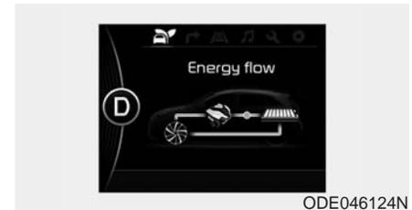
Vehicle is stopped with the Engine charging the hybrid battery.
