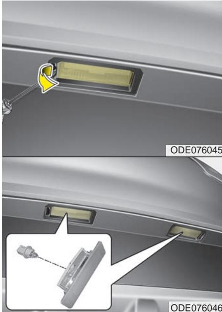
1. Using a flat-blade screwdriver, gently pry the lens cover from lamp housing.
