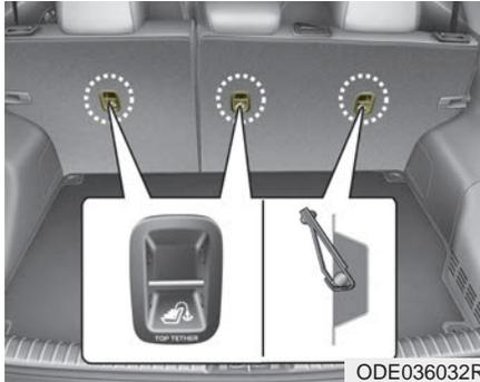
First secure the child restraint with the LATCH lower anchors or the seat belt. If the child restraint manufacturer recommends that the top tether strap be attached, attach and tighten the top tether strap to the top tether seat anchor.
