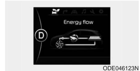
Engine power is used to move the vehicle. (Engine → Wheel)
