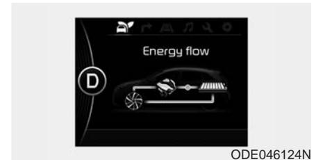
Vehicle is stopped with the Engine charging the hybrid battery.
