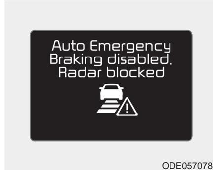
When the sensor is covered or the sensor lens is dirty with foreign substances, such as snow, rain, or debris, the AEB system may not be able to detect vehicles or pedestrians. In this case, a warning message will appear on the LCD display to notify the driver. Remove the foreign substances to allow the AEB system to function.
