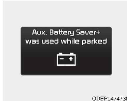
This message is displayed when the Aux. Battery Saver+ function has been completed when the vehicle is turned ON.
