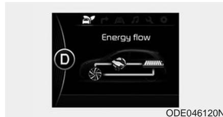
This mode means the vehicle has stopped.
