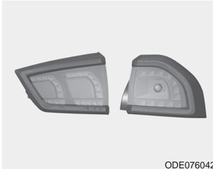
If the stop and tail lamp (LED) does not operate, have the vehicle checked by an authorized Kia dealer. The LED lamps cannot be replaced as a single component because they are part of an integrated unit. The LED lamps have to be replaced with the unit.
