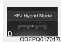
: The high-voltage (hybrid) battery and gasoline engine are used to charge the high voltage battery (hybrid) and drive the vehicle.
