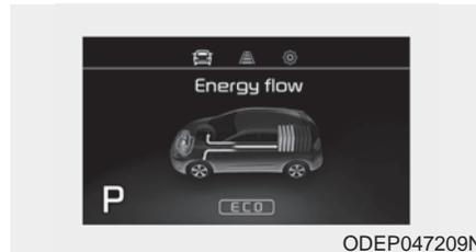
The vehicle is being slowed down by engine compression and regenerative braking. The hybrid battery is being charged by regenerative braking.
