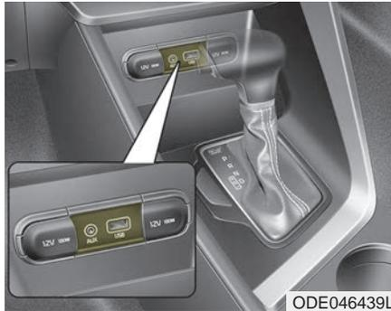
If your vehicle has an AUX and/or USB(universal serial bus) port, you can use the AUX port to connect audio devices and the USB port to plug in a USB device or iPod®.
