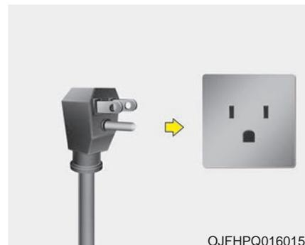
4. Disconnect the plug from the household electric outlet. Do not pull the cable when disconnecting the plug.
