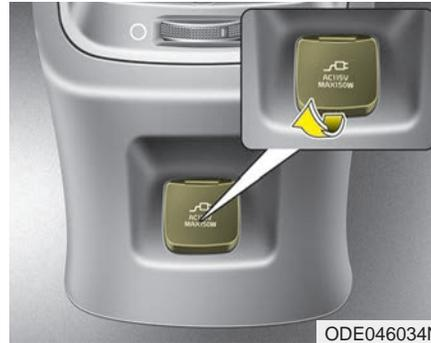
The AC inverter supplies 115V/150W electric power to operate electric accessories or equipment.
