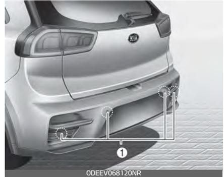
The sensing range and objects detectable by the back sensors (1) are limited. Whenever backing-up, pay as much attention to what is behind you as you would in a vehicle without a parking distance warning-reverse.
