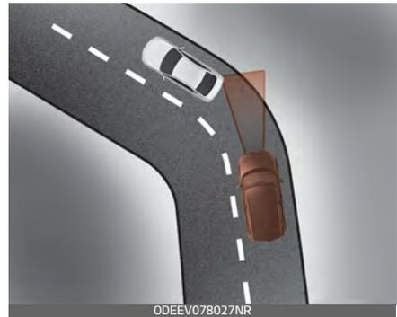
On curves, the smart cruise control system may not immediately detect a moving vehicle in your lane, and then your vehicle could accelerate to the set speed. Also, the vehicle speed will rapidly decrease when the vehicle ahead is recognized suddenly.
