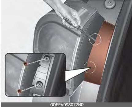
4. Remove the rear combination lamp assembly from the body of the vehicle.
