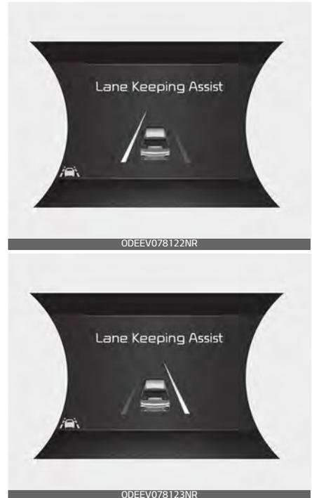
If the vehicle moves out its lane because steering torque for assistance is not enough, the lane indicator will blink.
