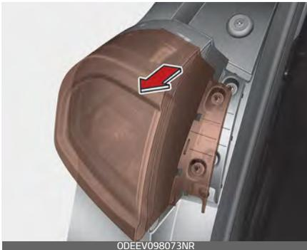
5. Disconnect the rear combination lamp connector.
