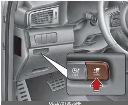
\* The charging inlet is locked during DC Charge regardless of the AUTO/LOCK mode. After charging is complete, the locked charging inlet is unlocked.
