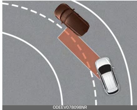
The BCW systems may not operate properly when driving on a curved road. In certain instances, the system may recognize a vehicle in the same lane.
