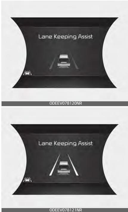
If the speed of the vehicle is over 40 mph (64 km/h) and the system detects lane markers, the color changes from gray to white.
