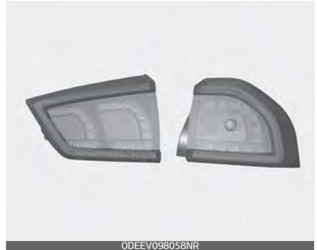
The LED lamps cannot be replaced as a single component because they are part of an integrated unit. The LED lamps have to be replaced with the unit.
