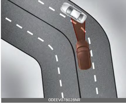
The FCA system may recognize a vehicle in the next lane when driving on a curved road.
