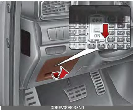
Always set the fuse switch to the ON position before using the vehicle. If you move the switch to the OFF position, some items such as audio and digital clock must be reset and transmitter (or smart key) may not work properly. When the switch is Off, the caution indicator will be displayed on the instrument cluster.
