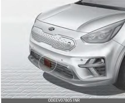
The sensor detects the distance to the vehicle ahead.
