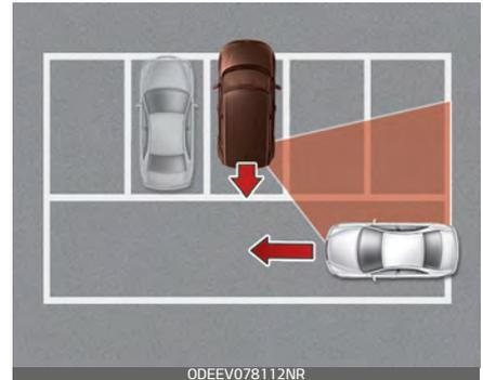
If the vehicle is parked rearward and the sensor detects the another vehicle in the rear area of the parking space, the system can warn or control braking.
