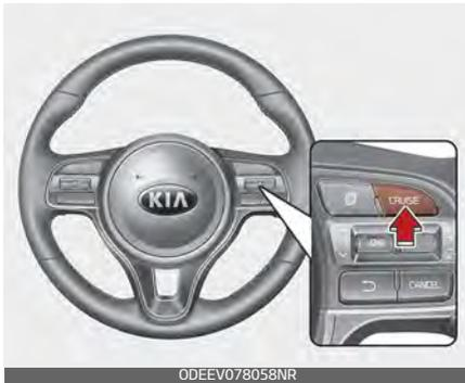
2. Accelerate to the desired speed. The smart cruise control speed can be set as follows:
