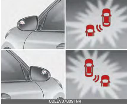
If a vehicle is detected within the boundary of the system, a warning light will illuminate on the outer side view mirror and the head up display (if equipped).
