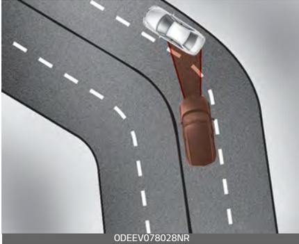
Your vehicle speed can be reduced due to a vehicle in the adjacent lane. Adjust your vehicle speed by depressing the brake pedal according to the road and driving conditions ahead.
