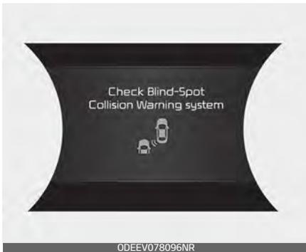
If there is a problem with the BCW system, a warning message will appear and the light on the switch will turn off. The system will turn off automatically. RCCW will not operate also if the BCW system turns off due to malfunction. Have your vehicle inspected by an authorized Kia dealer.
