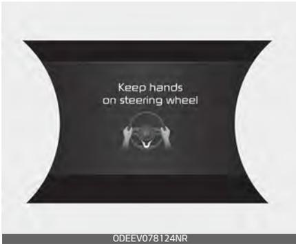
If the driver takes hands off the steering wheel for several seconds while the LKA is activated, the system will warn the driver.
