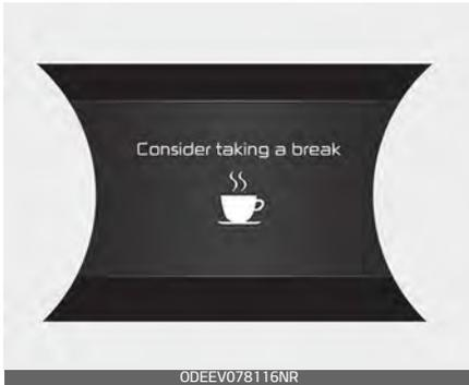
The Driver Attention Warning system will not suggest a break, when the total driving time is shorter than 10 minutes.
