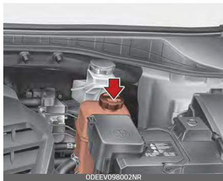
Do not remove the radiator cap when the motor compartment and radiator are hot. Scalding hot coolant and steam may blow out under pressure which may result in serious injury.
