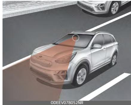
When the system detects the vehicle straying from its lane, it alerts the driver with a visual and audible warning, while applying a slight countersteering torque, trying to prevent the vehicle from moving out of its lane.
