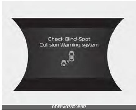
If there is a problem with the BCW system, a warning message will appear and the light on the switch will turn off. The system will turn off automatically. Have your vehicle inspected by an authorized Kia dealer.
