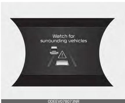
If the vehicle ahead (vehicle speed: less than 20 mph (30 km/h)) moves to the next lane, the warning chime will sound and a message will appear. Adjust your vehicle speed for vehicles or objects that can sud-
