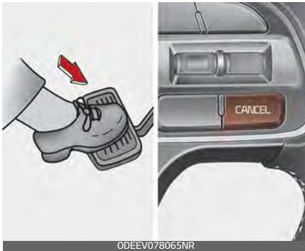
The smart cruise control is temporarily canceled when the brake pedal is depressed or the CANCEL button is pressed.
