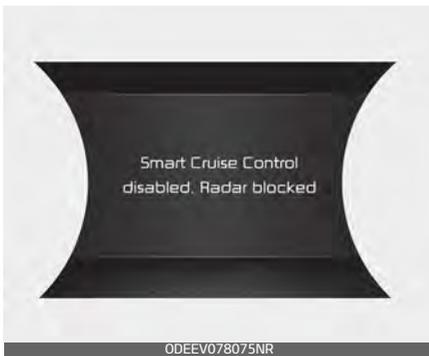
When the sensor lens cover is blocked with dirt, snow, or debris, the Smart Cruise Control System operation may stop temporarily. If this occurs, a warning message will appear on the LCD display. Remove any dirt, snow, or debris and clean the radar sensor lens cover before operating the Smart Cruise Control System.
