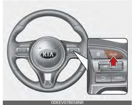
When the Smart Cruise Control System is not needed, press the [CRUISE] switch and deactivate the system.
