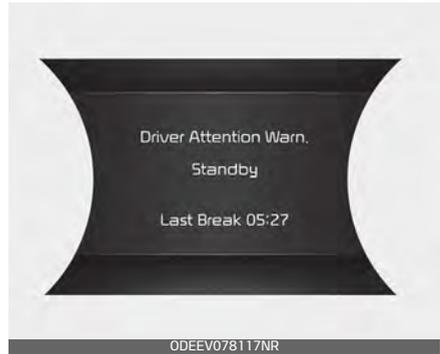
The last break time is set to 00:00 and the driver's attention level is set to 5 (very attentive) when the driver resets the Driver Attention Warning system.
