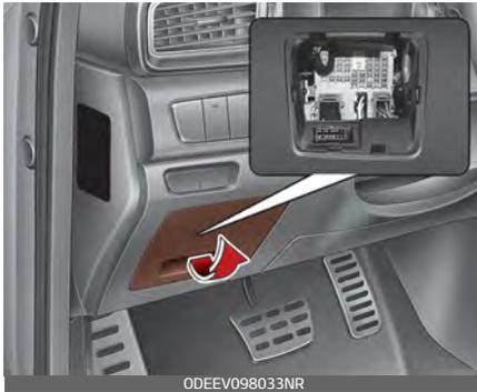
If the switch is located in the "OFF" position, a caution indicator will be displayed in the cluster. To identify the location of a specific fuse, please refer to the inside of the fuse panel cover and the description list in this section.
